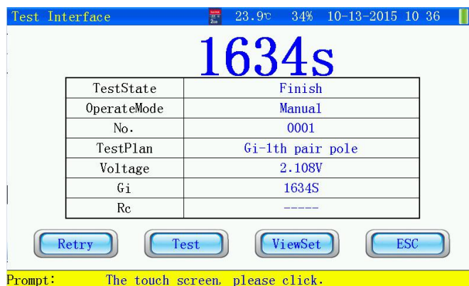
Fig. 3.3.1-3 More than 2 poles and connection strip test on voltage and battery conductance
